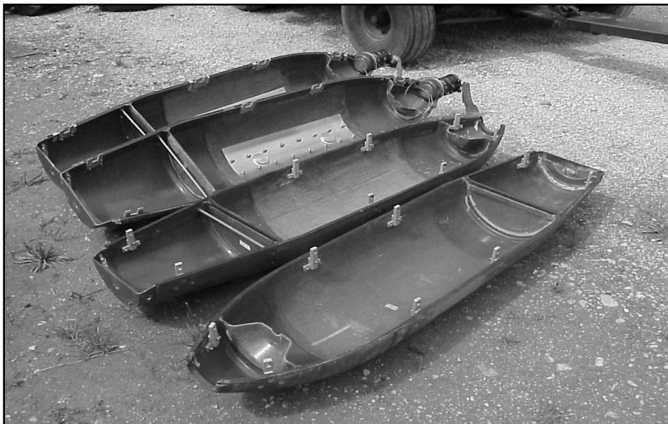
Figure D-8. MK129 casing rigged with detonation cord prior to packing
