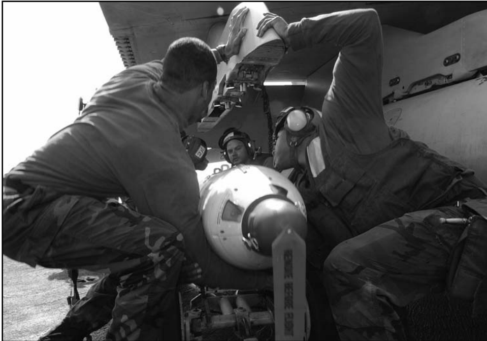
Figure D-18. Technicians attach a PDU-5/B LDS to an FA-18 Hornet
