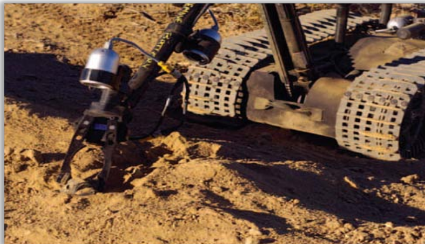
Figure 3. Talon Ordnance Disposal Robot Preparing to Unearth Simulated IED
